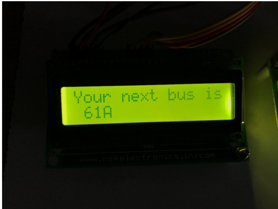
Fig 8.7 LCD to display detect the arrival of one bus and prompt the wait for another
